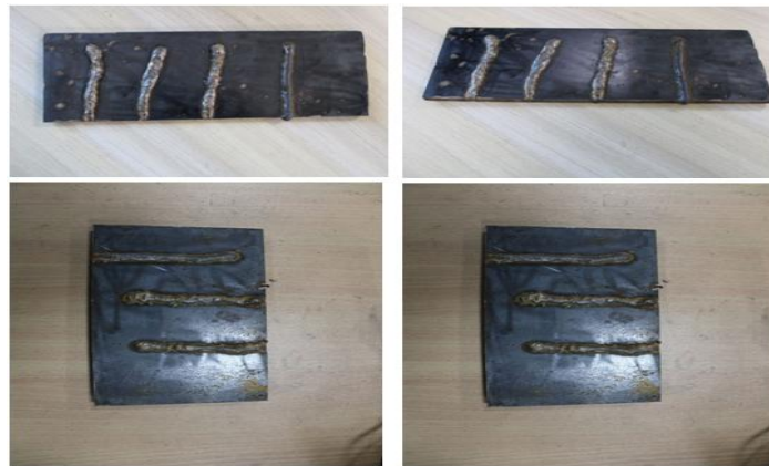
Figure.1 Weld beads achieved during the welding process
