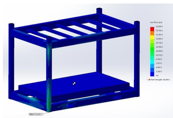
Figure 10. Resultant von Mises stress plot of the lifting frame.
