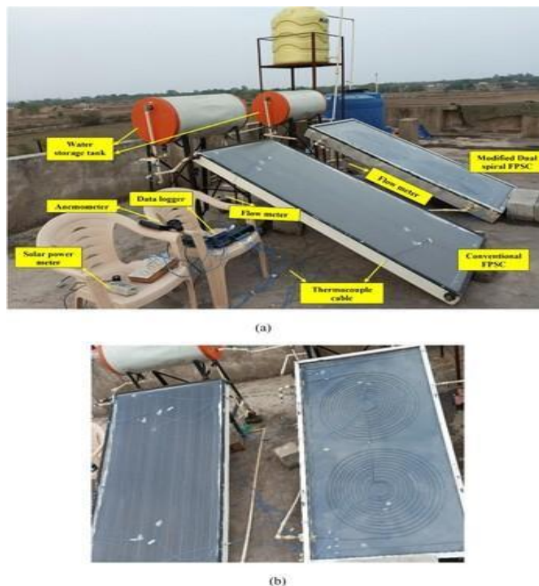
Fig.1. Experimental Setup of the Conventional and Modified Flat Plate Solar Collectors
