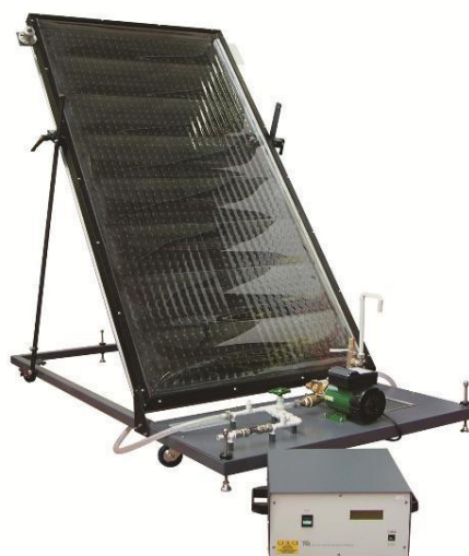
Fig.2. Experimental Setup of a Solar Thermal Collector with Tracking and Measurement System
