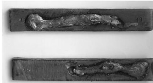
Fig. 10. Specimens with test beads obtained by wet underwater welding conditions with the use of covered electrodes
