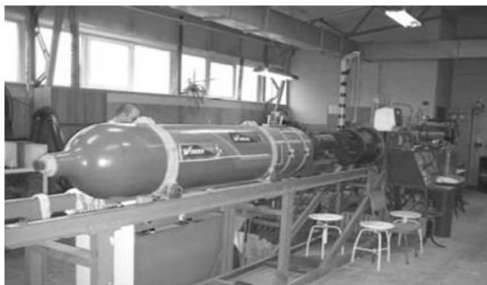
Fig. 13. Test facility for simulating underwater welding on high depths
