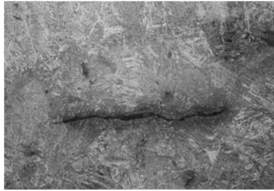
Fig. 5. Microphotograph of the cold crack in the bainite structure of heat affected zone [18]
