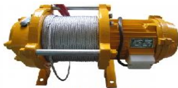
Figure (a) Hoist motor
