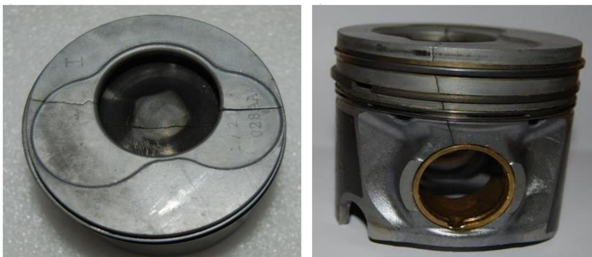
Fig. 1. 2. A crack on the piston pin: a) cracked piston head; b) cracked piston skirt
