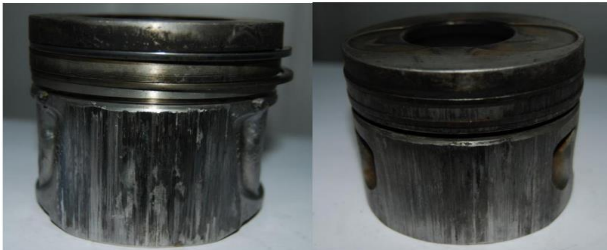
Fig.1.1. A piston skirt seizure
