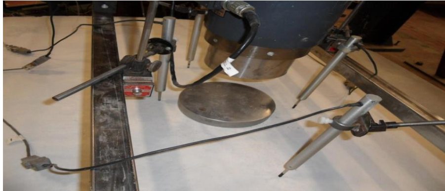
Figure .5 – Another view for experimental setup for punching test of lining segment
