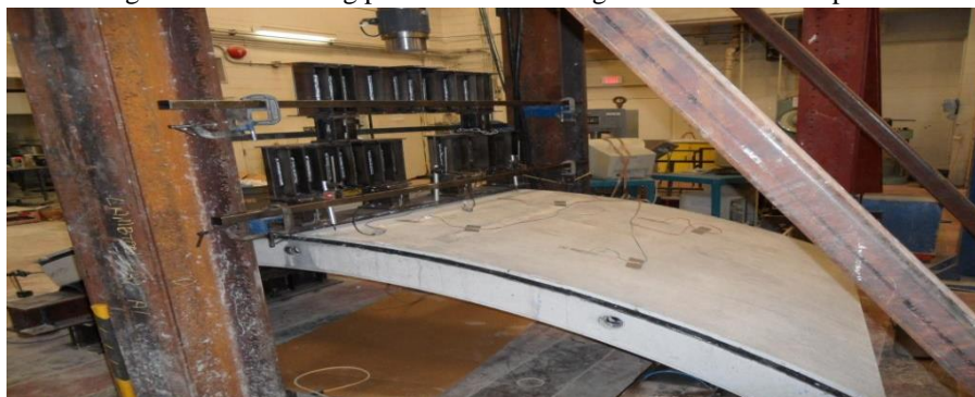
Figure .3 – Another view for experimental setup for flexural testing of lining Segment http:// www.ijrtsm.com © International Journal of Recent Technology Science & Management
