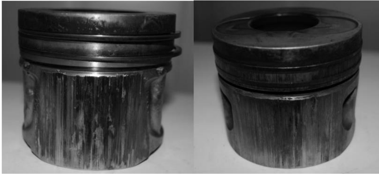
Fig.1.1. A piston skirt seizure
