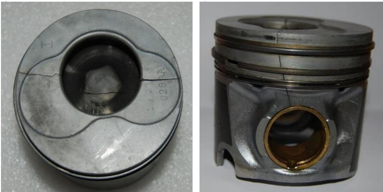
Fig. 1. 2. A crack on the piston pin: a) cracked piston head; b) cracked piston skirt
