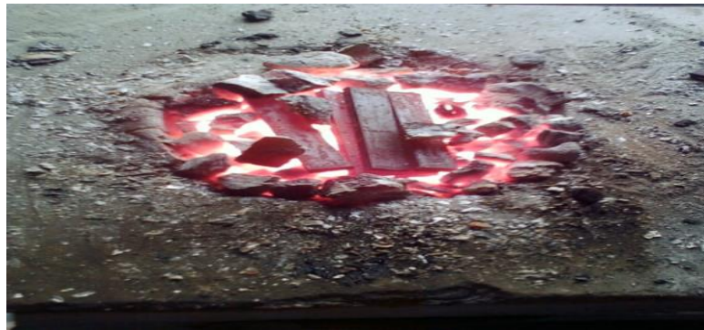
Fig.10 Hardening Process of Mild Steel in Open Hearth Furnace
