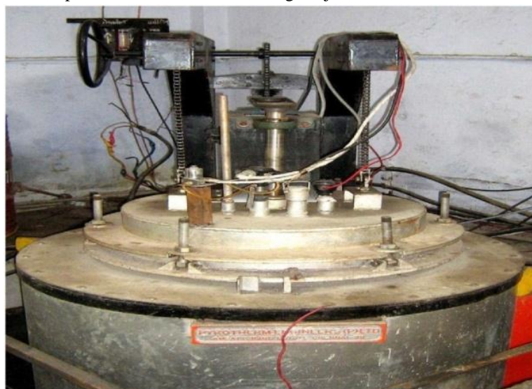
Fig. 1 Gas carburizing furnace
