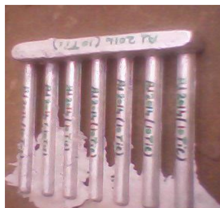
Figure.5.1: Melting facility and castings of Al-TiC Composites
