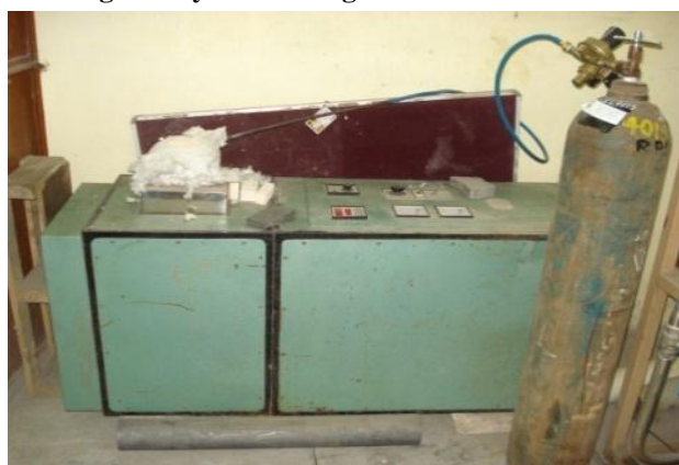
Figure.5.1: Melting facility and castings of Al-TiC Composites
