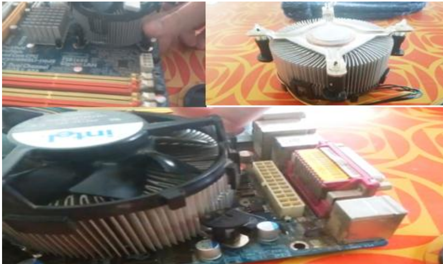
Figure 1.1: Heat sink CPU arrangements
