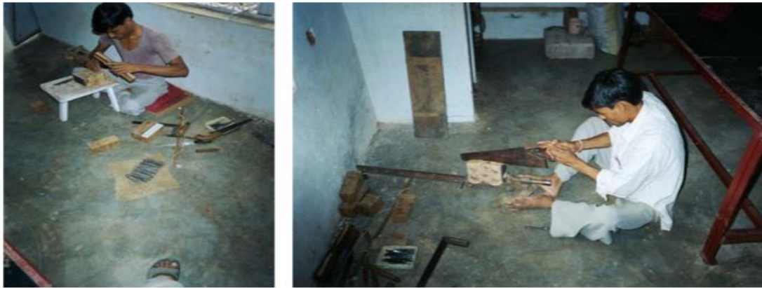
Fig. 3.3: Wooden block making process 1, 2.
