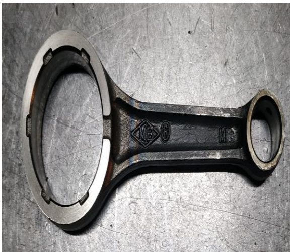
Fig 4.1 Front View of as built connecting rod of Bajaj discover 150cc model
