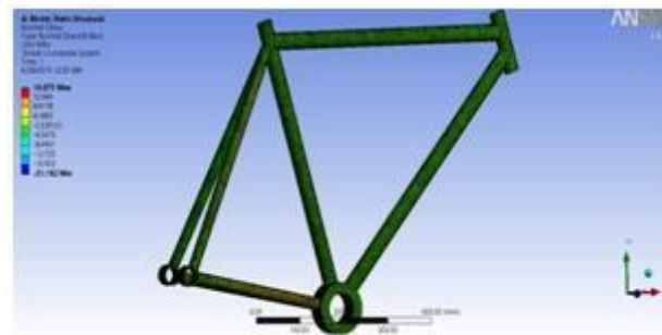
Figure 13: Rear wheel braking
