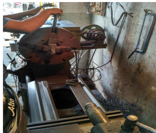
Fig 1.2 Making tool on lathe machine for FSW
