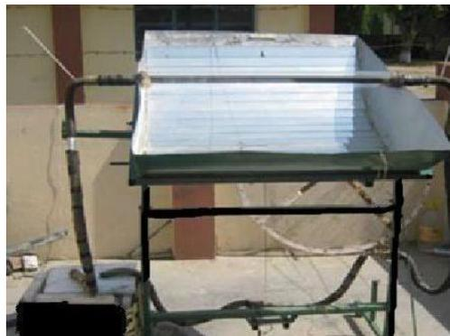
**Fig-2 Parabolic trough collector system**
